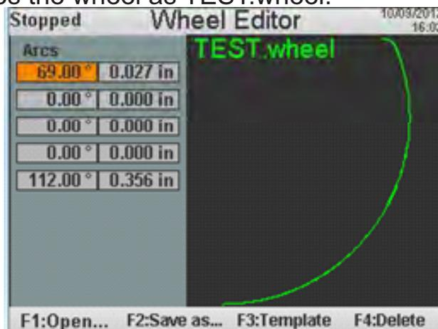
Once the wheel has been designed it can be opened and edited by selecting it in the wheel editor. Changes made to any wheel open in the editor can be saved by pressing the Save button on the HMI. After saving TEST.wheel, the selection becomes available for use in the wheel catalog as shown below:
