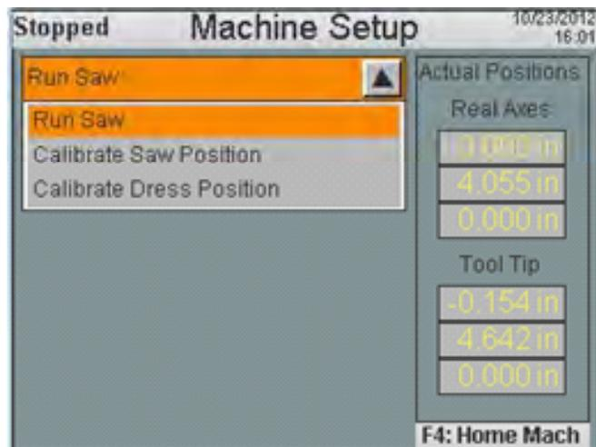
An initial calibration of the grinding head in relationship to the saw tip position and the dressing pellet is made when the machine is originally commissioned. These initial positions are overwritten when a wheel is installed and the grinding wheel is set up on a tooth. The operator should not have a need to use the calibrate options.
