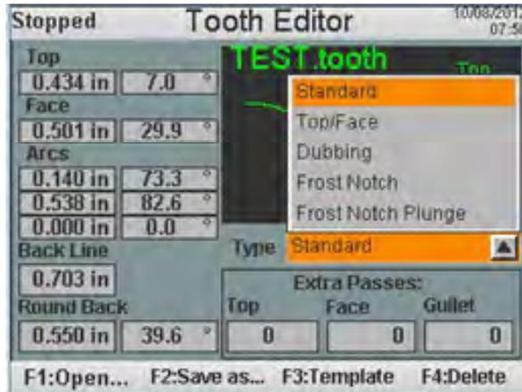
To save our above example, press the F2 button to open the file options. The up/down arrows allow selection of previously designed teeth should the operator want to use an existing tooth name and overwrite a tooth that was previously made. To do that toggle through the options until your choice is displayed in the highlighted
