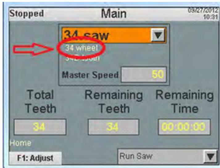
Pressing F1 opens the editor where wheels are created and modified. If no wheel has been opened since the last power-up, there will be no name displayed and all the values will read zero when the editor is opened
