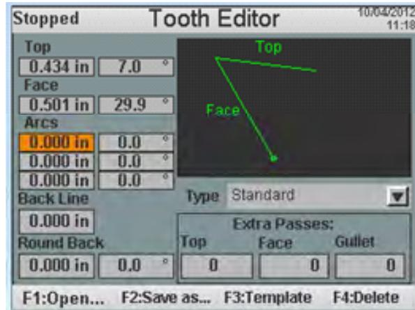
Each tooth is allowed up to 3 arcs to form the gullet shape. The first arc in the above example has a radius arc distance of 0.140 at 73.3°. These values must be entered into the first arc position. **Caution: Placing values in position two or three while leaving zeros in the position above it could cause the grinding wheel to move directly into the gullet!!** After the first arc values are entered the
