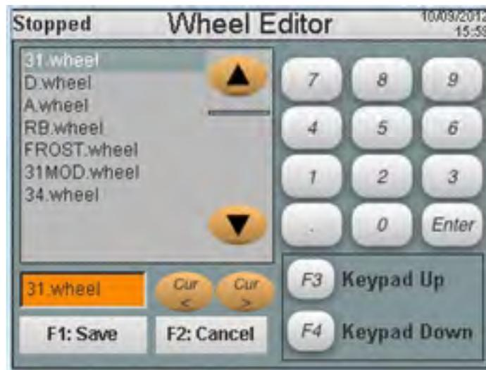
To save the new wheel with **anewname** press the right arrow key once to place the cursor inside the orange box. With the right/left arrow keys place the cursor just to the left of the .wheel characters. Press the F4 key once to change the number pad to letters and press the delete key until only .wheel is remaining. The editor should now look like this:
