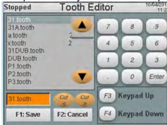
To make a new tooth name, any existing tooth can be renamed and saved without being overwritten. Notice that 31.tooth is highlighted in orange in the above example. Since that's not what we want to call our new tooth we are going to change the name in the field and save it with a new name. Pressing the right arrow key places a cursor inside the field. Move the cursor until it is just to the left of .tooth
