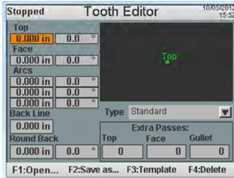
If a tooth has been not opened since the last power-up, there will be no name displayed and all the values will read zero. Begin designing a tooth by entering the desired tooth values developed in a cad file. As the values are entered into the editor the tooth shape is drawn on the editor screen. Below is an example of how the tooth shape develops as the values are entered from the CAD diagram.
