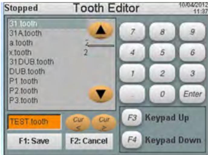
Pressing F1 now saves the newly designed tooth as TEST.tooth and makes it available in the Tooth Catalog for viewing and for selection in the Saw screen menu.
