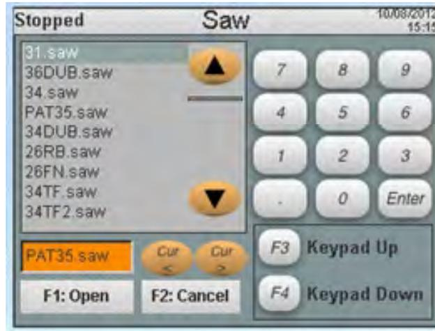
**F2:Saveas** – Opens options for saving the saw program. Toggle through the selections with the up/down arrow keys and press F1 to save the saw as the .saw file highlighted in orange.
