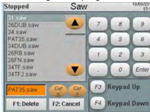
Pressing F1 in the above example will bring up a pop up box that asks if you're sure you want to delete PAT35.saw. When a saw program is deleted the operator must select and load a saw program from the Main page. Wheel selection for saw programs: The wheel for each saw program is loaded when the saw program is opened and displayed below the saw name:
